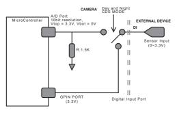
External CDS is only active when day and night mode is set to EXT Mode in the OSD. CDS: External device to control day and night status
